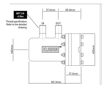
Designs incorporating Klaran WR should use the reactor in one of the two acceptable orientations to ensure performance meets specifications. Failing to do so may result in inadequate disinfection performance or damage to the Klaran WR.
